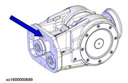
The hole is available on robots introduced with Axis Calibration.
