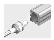
• Place the piston flat against the front side of the cylinder barrel and insert the lip ring into the cylinder barrel by tilting and turning it slightly.
