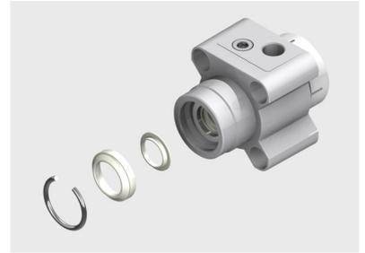
26. Apply a thin film of the grease included in the set of wearing parts on the new buffer seals on the front side facing the sealing surface.
