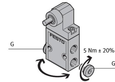
The plug screw (G) can optionally be screwed in to the left or right in connection 2.
