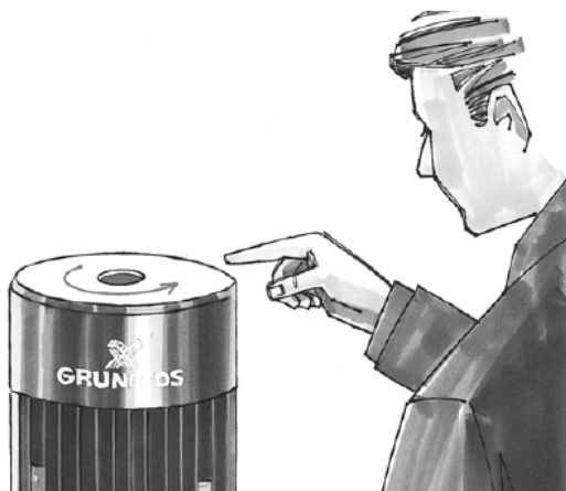
Checking rotation of the pump
