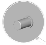
Figure 5-6 Earth Grounding lug
