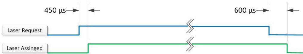
Laser Request signal Vs Laser Assigned signal
