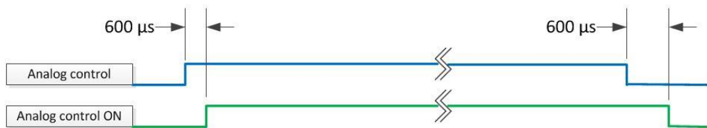
Analog Control signal Vs Analog Control On signal
