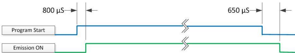
Program Start signal Vs Emission ON signal for program 0
