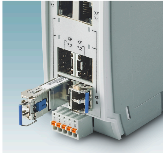
Figure 4-27 Inserting the SFP modules (example)
