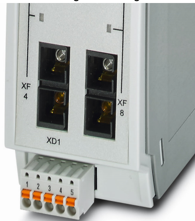
Figure 2-1 Integrated fiberglass transceivers with an SC pin connector pattern
