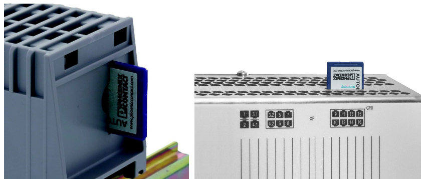
Figure 4-28 Position of the SD card slot on versions 20xx–23xx (left), versions 24xx and 25xx (right)
