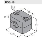
6901320 Mounting clamp for smooth and threaded barrel sensors; material: Polypropylene
