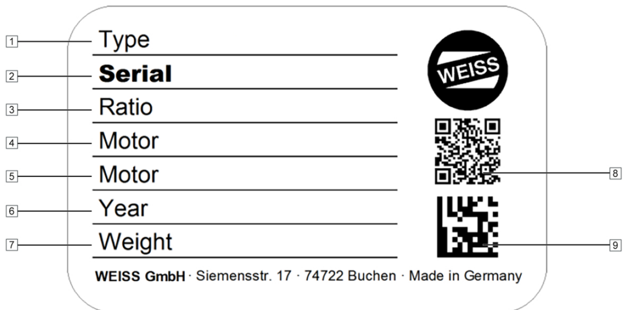
Figure 1: Example of nameplate
